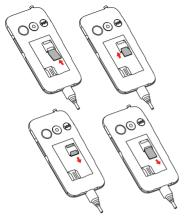
Place the SIM card with the chip facing downwards and slide it into its housing. Make sure that it is correctly inserted. To remove the card, press and slide it out.
